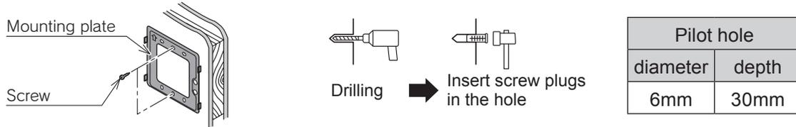
\*Use the attached screw plugs if the mounting plate is fixed by screws to tile, concrete, and mortar wall.
