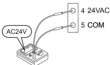
[Fig. 9] Voltage of 3way mixing valve (control)
