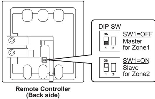
Note1: Communication error will occur if 2 Master Remote controllers and 2 Slave Remote controllers are connected.
