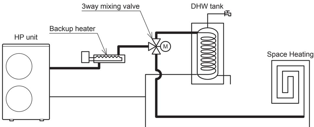
A parameter defines if the Backup heater can be enabled or disabled, and the “Type of function”:
