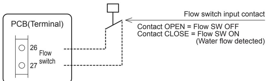
At Start-up, the compressor will not be turned ON unless the flow switch is CLOSED (water flow detected).
