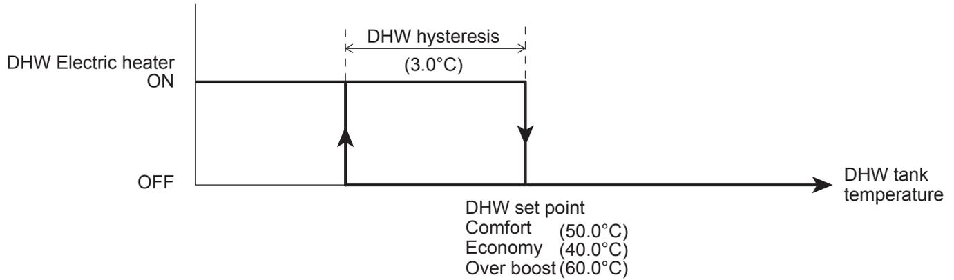
If the Par3102=2 (Heater only), the heat pump produces hot or cool water for the system and the hot water will be heated by the electrical heater only.
