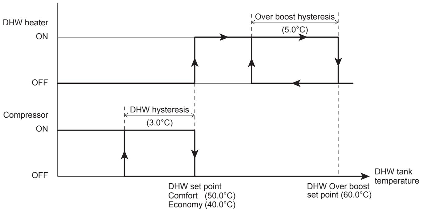
The DHW set point is reached (Comfort or Economy) using the compressor, the Over boost set point will be achieved with the DHW heater only and the HP unit will change over to the system.
